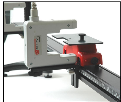
Dynamics equipment for studying Newton's Second Law of Motion
